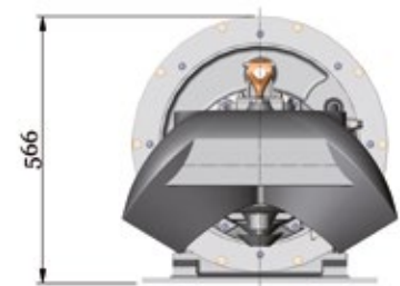
OUTBOARD VIEW OF MJP ULTRAJET UNIT
