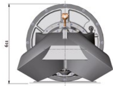
OUTBOARD VIEW OF MJP ULTRAJET UNIT
